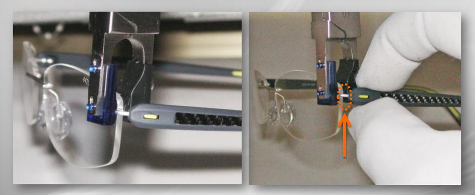
Hold lens fixation in position with mounting pliers. Open temple completely. Enclose temple edge firmly and adjust inclination on titanium side part in requested direction.
