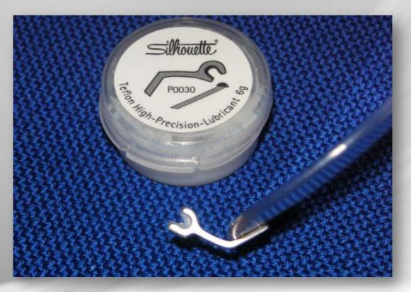
After cleaning grease inside loop of hinge with Teflon High Precision lubrication mount temple.
