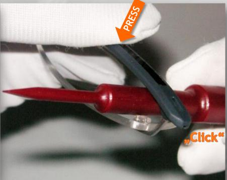
Place disassembly tool where lens and temple meet as shown.
